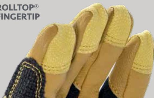
**Attributes** - No seams across the fingertip. Palm fabric rolls up and over fingertip. Fabric panel typically has an hourglass shape to create a form-fitting fingertip.
